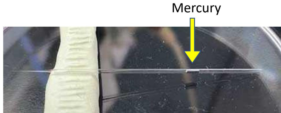
Glass pipette filled with mercury
